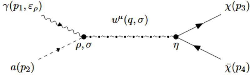
**Fig. 1.** The Feynman diagram for  $a\gamma \rightarrow \chi\bar{\chi}$  process via radion.
