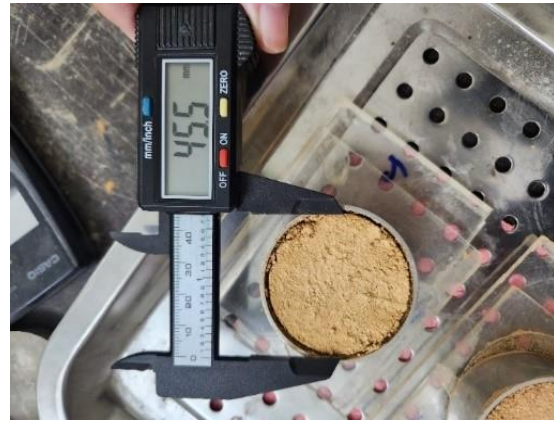
Figure 5. Measuring the diameter of the SC specimen
